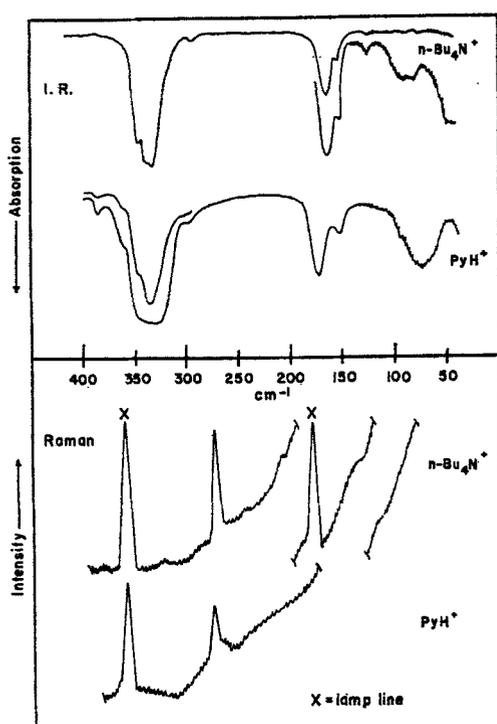
FIGURE 1. Infrared and Raman spectra of butylammonium and pyridinium salts of  $\text{Re}_2\text{Cl}_8^{2-}$ . Infrared spectra recorded on Nujol mulls. Raman spectra recorded on solid samples using  $4765\text{ \AA}$  line of argon ion laser.
