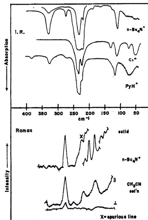
FIGURE 2. Infrared spectrum of  $\text{Cs}_2\text{Re}_2\text{Br}_8$ . Infrared and Raman spectra of butylammonium and pyridinium salts of  $\text{Re}_2\text{Br}_8^{2-}$ . Infrared spectra recorded on Nujol mulls. Raman spectra on solid and  $\text{CH}_3\text{CN}$  solution using  $6328\text{ \AA}$  line of He-Ne laser.
