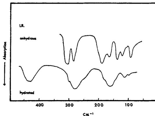
FIGURE 3. Infrared spectra of  $\text{K}_4\text{Mo}_2\text{Cl}_8$  and  $\text{K}_4\text{Mo}_2\text{Cl}_8 \cdot 2\text{H}_2\text{O}$ , recorded on mineral oil mull specimens.
