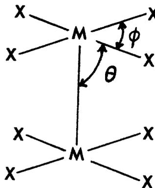
FIGURE 5. The  $\text{M}_2\text{X}_8$  skeleton ( $D_{4h}$  symmetry) with the bond angles  $\theta$  and  $\phi$  defined.
