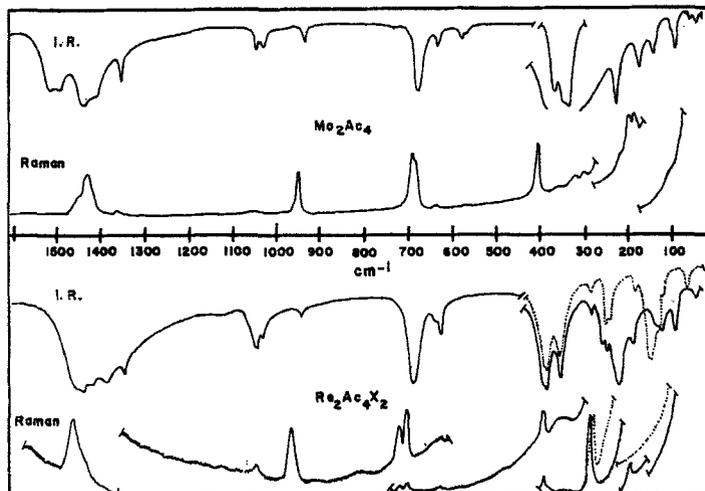
FIGURE 4. Infrared and Raman spectra of rhenium and molybdenum acetates. Infrared spectra recorded on KBr pellets and Nujol mulls. Raman spectra recorded on solid samples using 6328 Å line of He-Ne laser. Solid trace in  $\text{Re}_2\text{Ac}_4\text{X}_2$  spectra is for  $\text{X}=\text{Cl}$ ; broken trace is for  $\text{X}=\text{Br}$ .
